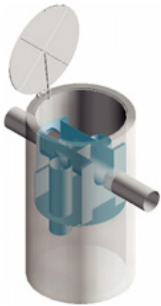
Fig. 11 Dual-vortex hydrodynamic separator for stormwater treatment.
