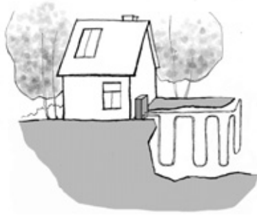
Figure 8: An illustration of a vertical, closed loop ground source heat pump.
