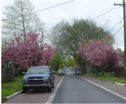
Fig. 2 Local 2-lane Street with pervious parking strips.
